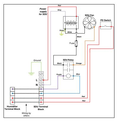
Illustration 7 - Wiring for SDU Model at 208V, 480V or 600V (1ph)
