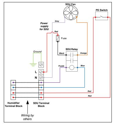
Illustration 6 - Wiring for SDU4-1 Model at 120V or 240V (1ph)
